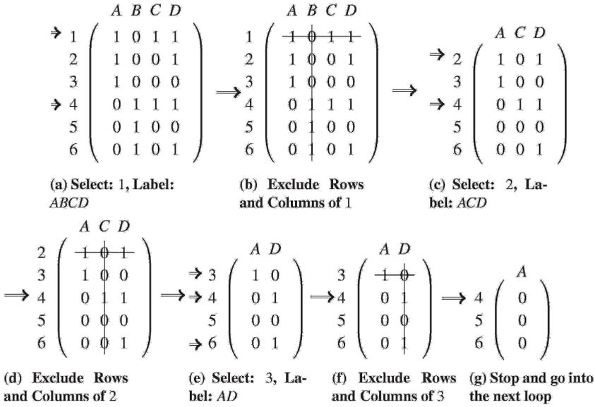
Fig. 4: Procedure of Algorithm 1
